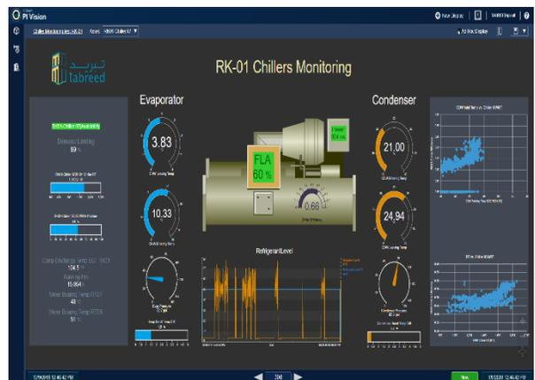
Figure: Chiller Monitoring Screen
