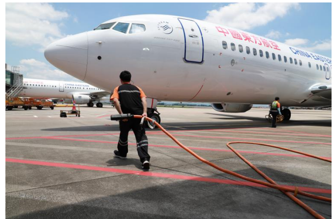
Figure 5 Using APU replacement facilities
