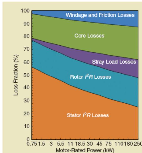
FIGURE 2. Typical fraction of losses in 50-Hz, in four-pole squirrel cage Induction Motors (de Almeida, Ferreira, & Fong, 2011)
