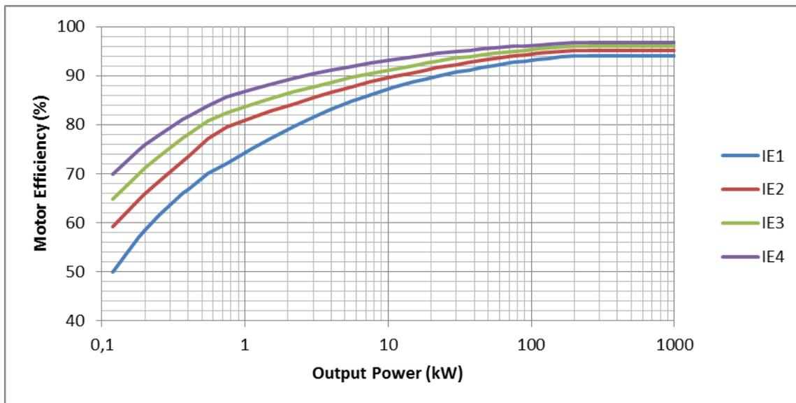
FIGURE 3. Efficiency levels in the 2014 version of IEC 60034-30-1 (example shown is for 4 pole motors, 50 Hz)
