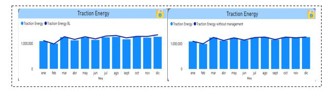
The first graph shows the actual traction energy consumption (bars) compared with the traction energy provided by the generated baseline (line). The second graph shows the actual traction energy consumption (bars) and compares it with the traction energy if fleet management had not been carried out.
